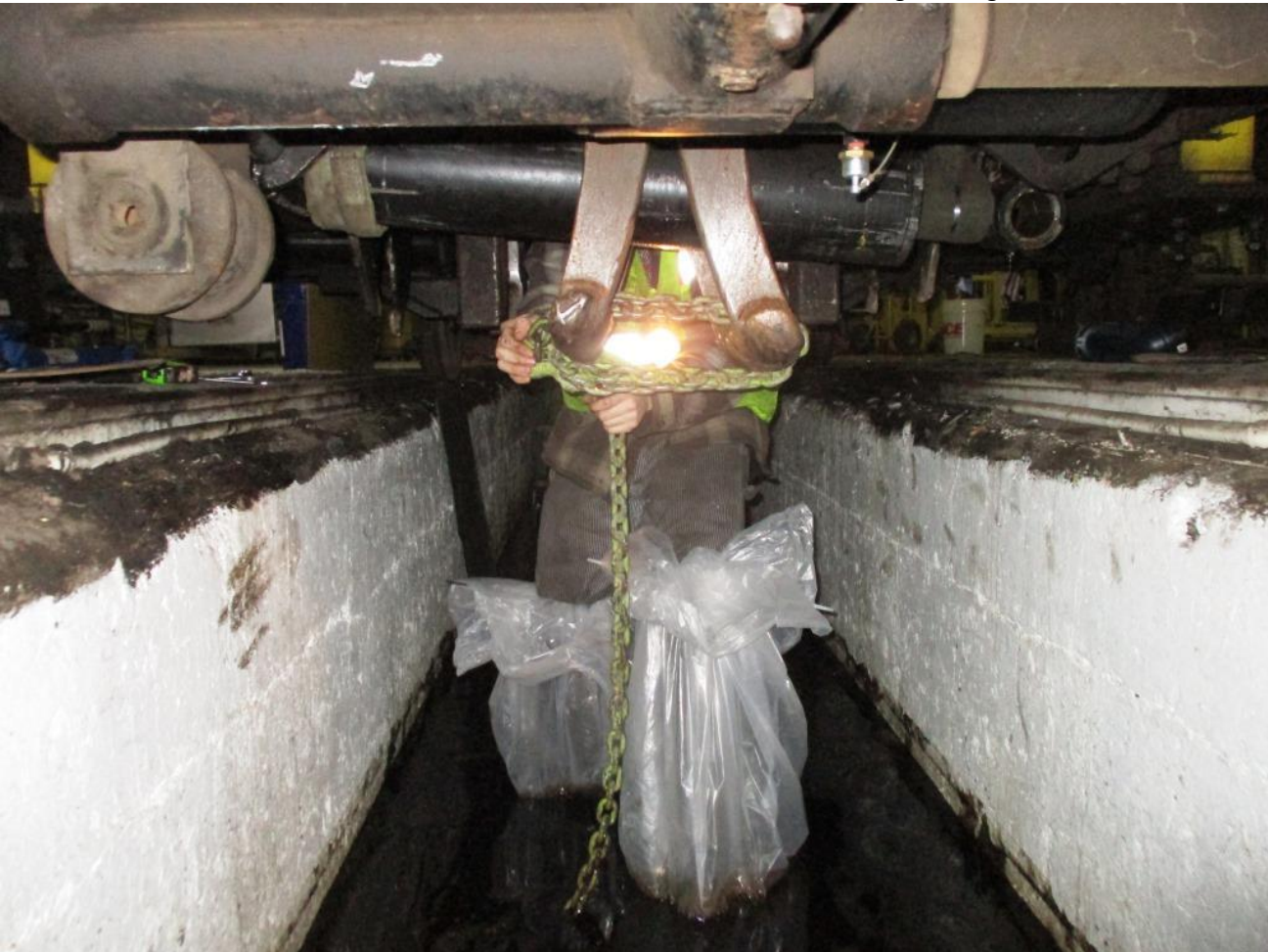
But, they have a practical purpose, as well, as Matt demonstrates as he chains the tie-shear's kickers into place
