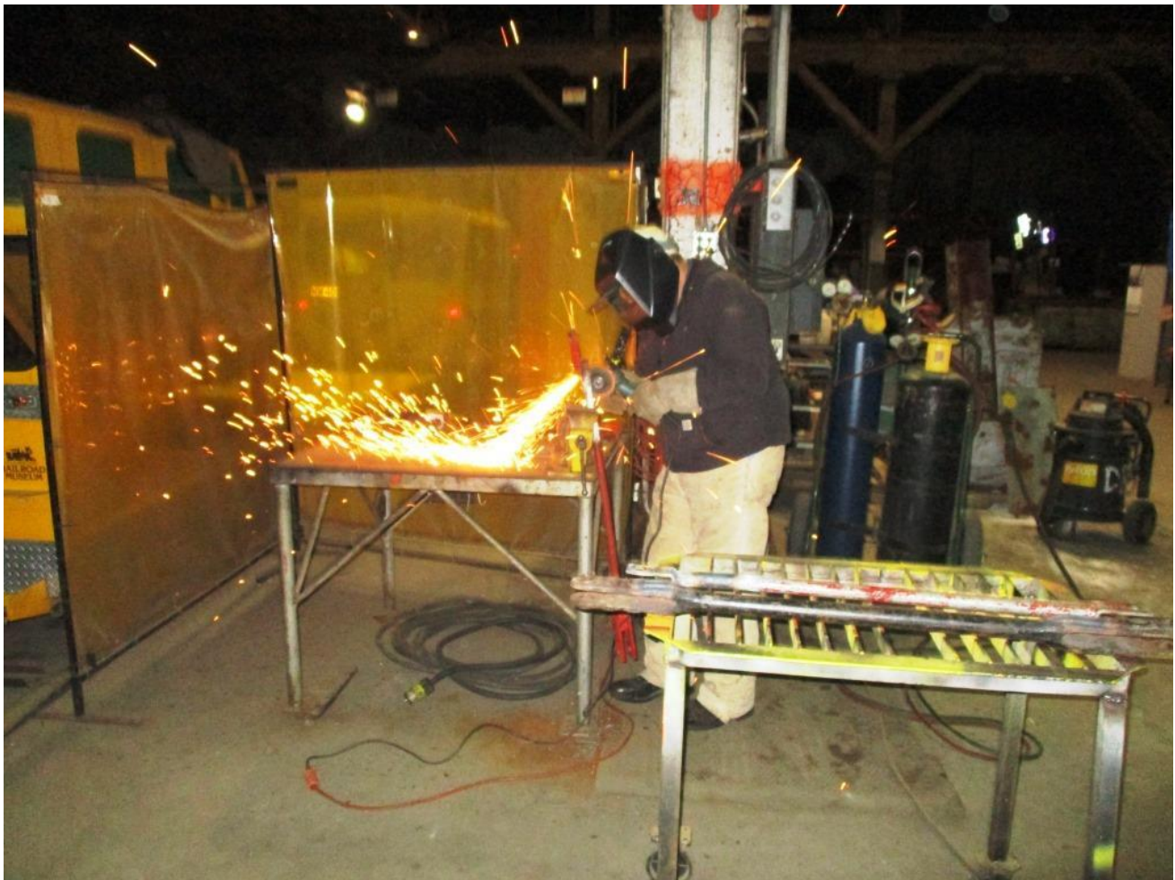
Cliff grinds the old, broken welds off of a draw-bar
