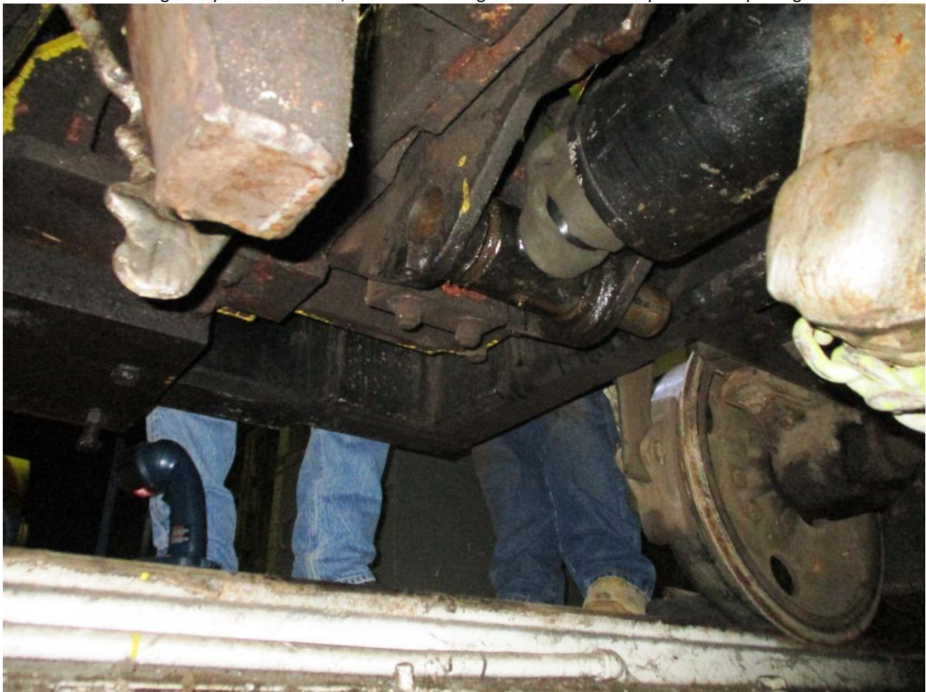
Under the tie-shear, the rather hefty hydraulic cylinder and pin that need to come out
