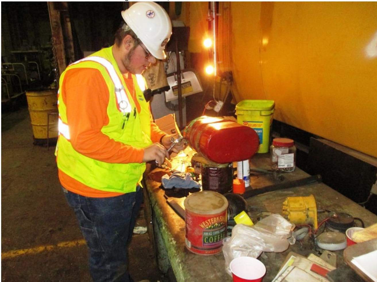
Chris H. installs a new valve on the derrick-car's gas-tank
