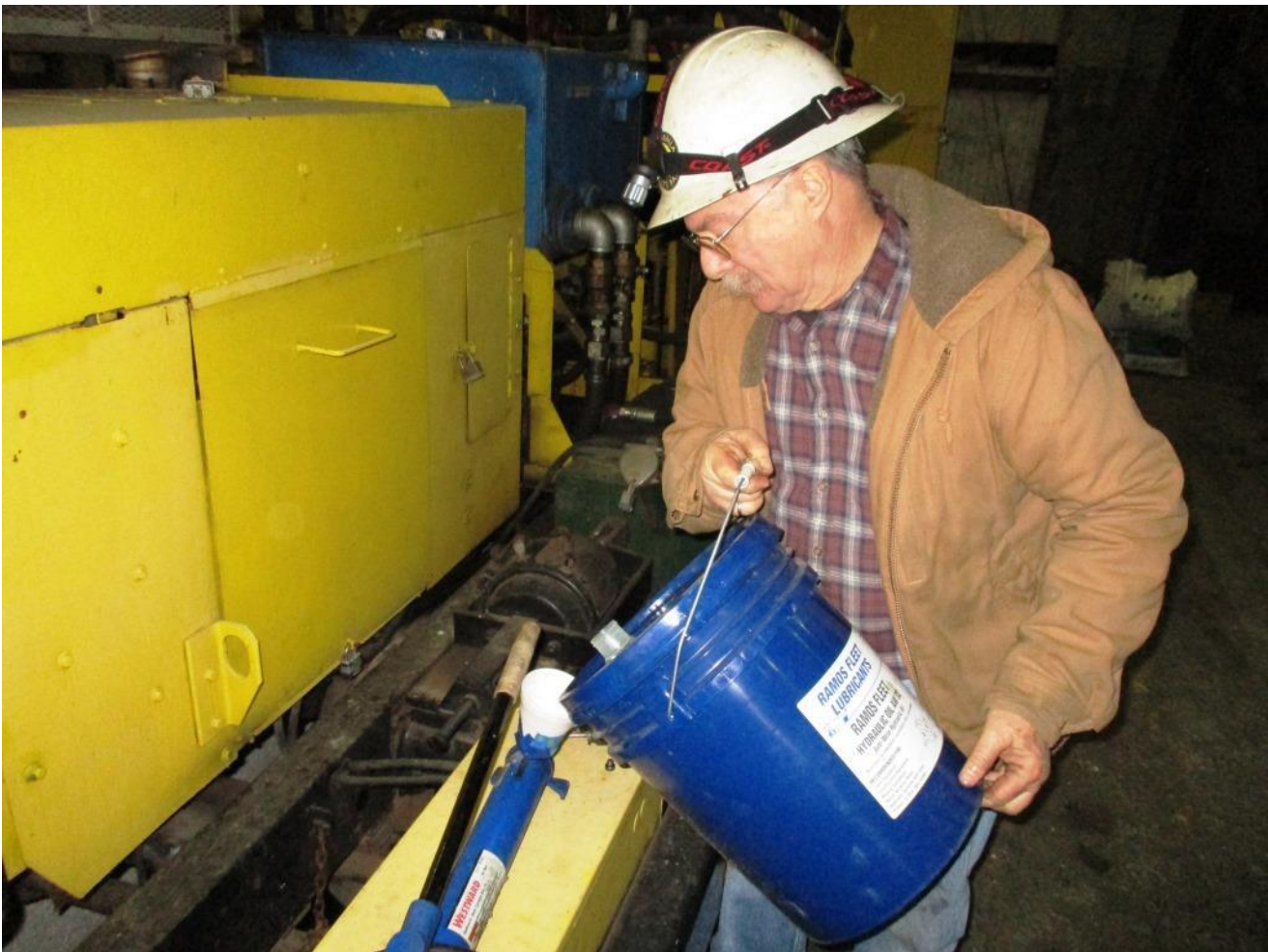
Mike H. pours hydraulic fluid into the Porta-Power using "MacGyver" Joe's improvised funnel
